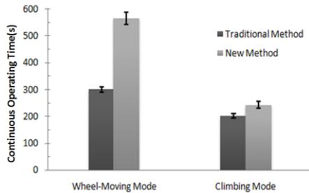
Figure 17. Result of the continuous operating time in the power consumption test. These results are briefly compared with traditional method for designing mobile platforms and the new method
